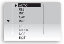
**AUTO MODE:** Select AUTO mode (AM sign appears at the left bottom corner of display) for automatic measurement of inductance, capacitance or resistance.
