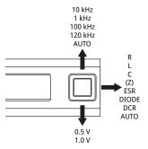
Note: To avoid errors do not use the Quick Controls during component measurement. UP – change test ranges
