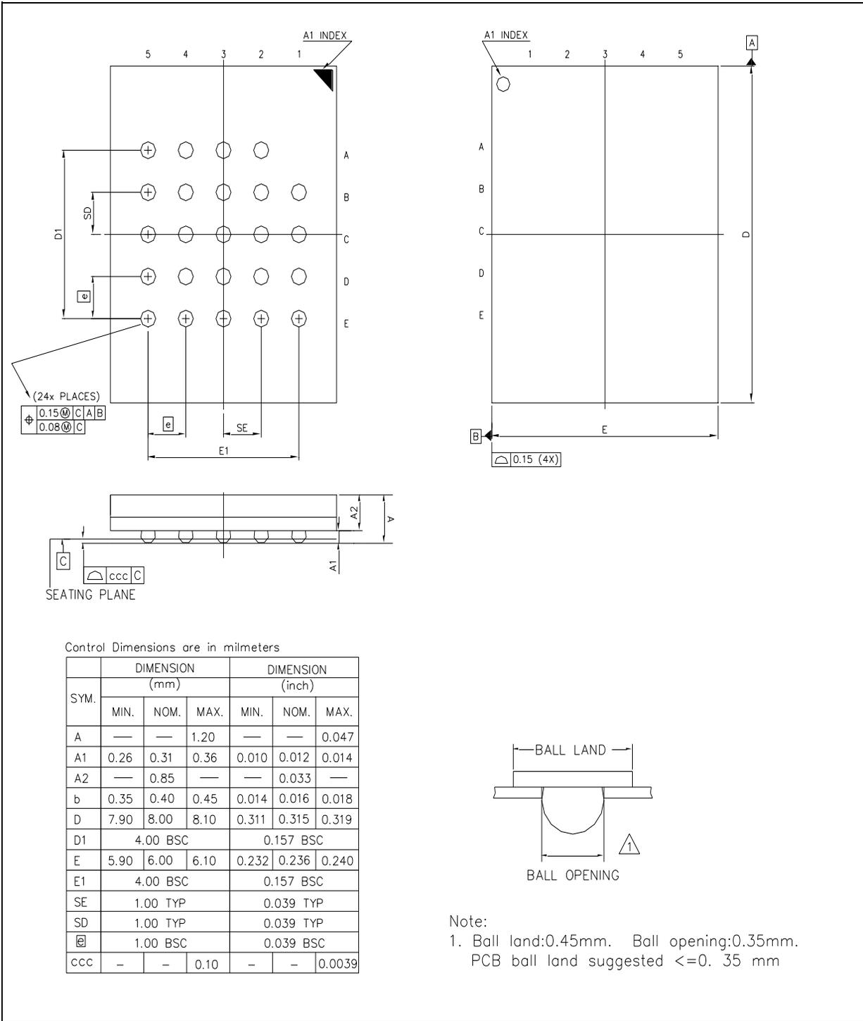
Control Dimensions are in millimeters
