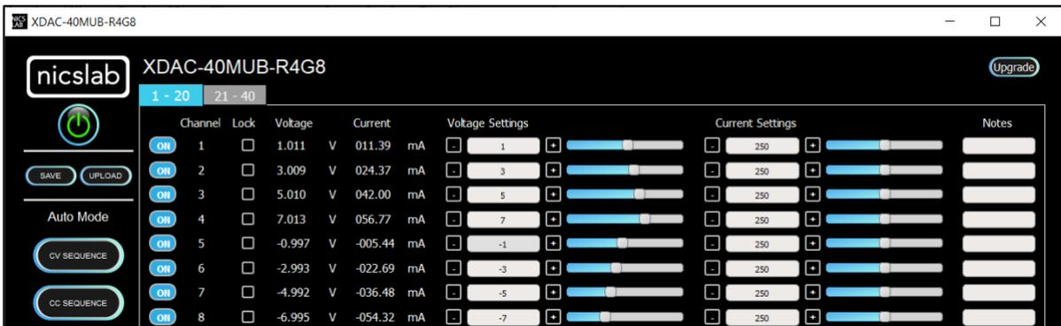
Note: When you upload CV mode, the current setting slider values automatically show 2184.50 bits to open the current flow from the supply. You may adjust this to match your requirements.
