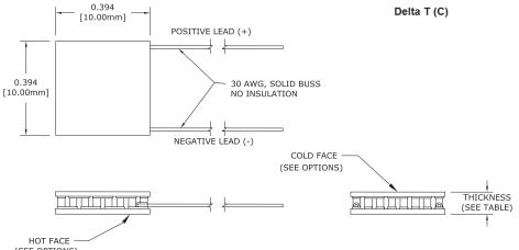
Ceramic Material 96% Alumina Ceramics Solder Construction: 138°C BiSn
