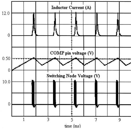
Figure 6. Hiccup Overcurrent Protection
