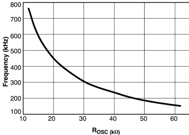
**Figure 8. Switching Frequency**
