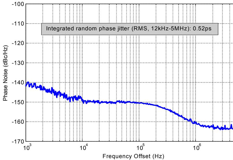
**Figure 3. Phase Noise, 10 MHz, 3.3V, LVC MOS Output**
