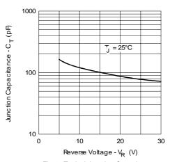
Fig. 3 - Typical Junction Capacitance Vs. Reverse Voltage
