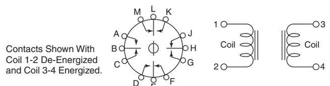
Contacts Shown With Coil 1-2 De-Energized and Coil 3-4 Energized.
