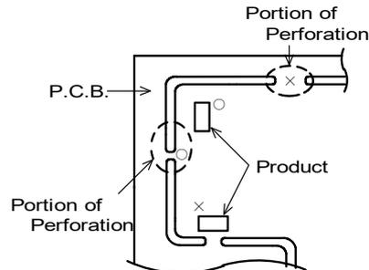
Products shall not be arranged on the line of a series of holes when there are big holes in P.C.B. (Because the stress concentrates on the line of holes.)
