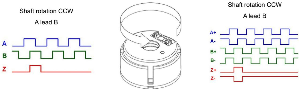
Figure 7: Example wave form for CCW rotation
