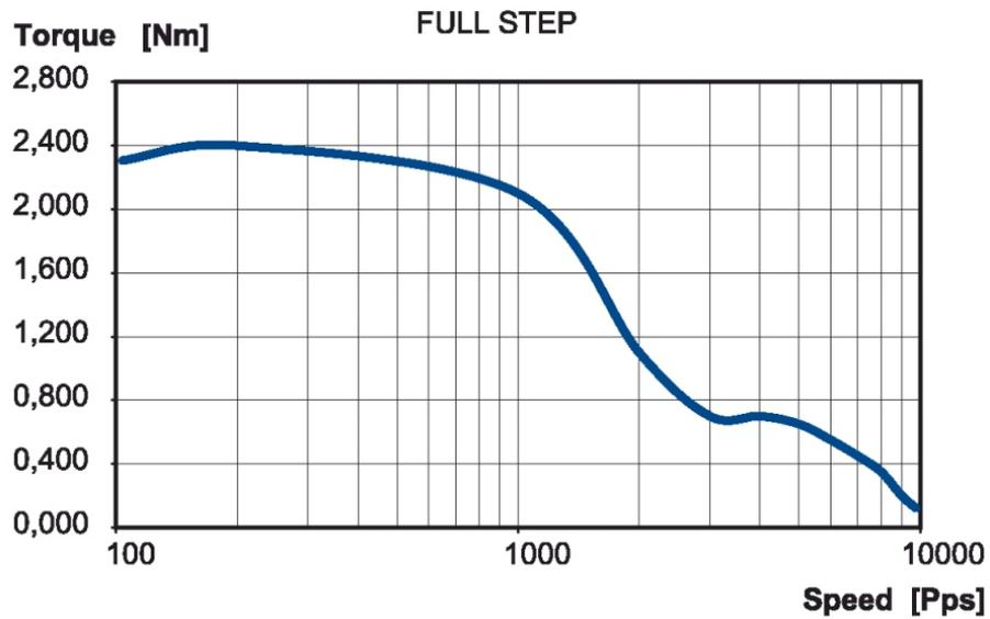
Figure 2: QSH6018-86-28-310 velocity vs. torque characteristics
