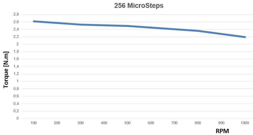
Figure 4: QSH6018-86-90-300 velocity vs. torque characteristics
