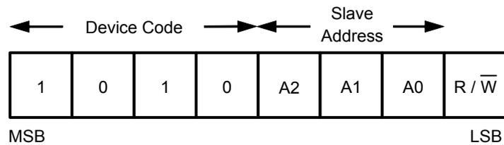
**Figure 11 Device Address**
