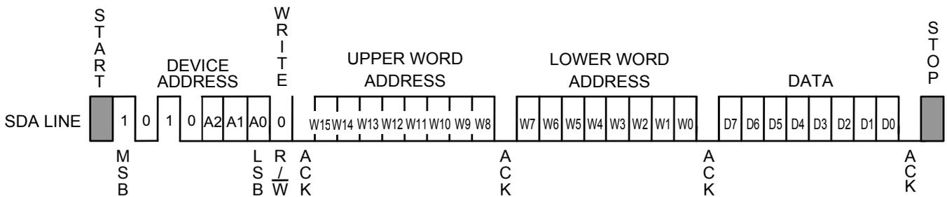
**Figure 12 Byte Write**
