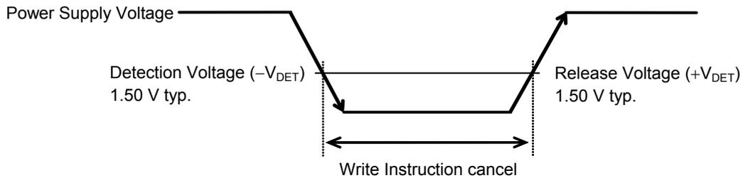
**Figure 19 Operation during Low Power Supply Voltage**
