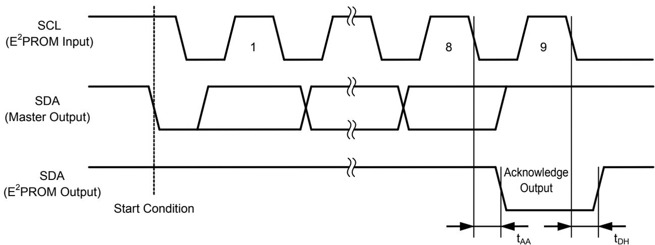
**Figure 10 Acknowledge Output Timing**
