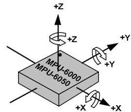
Orientation of Axes of Sensitivity and
