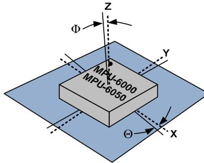
**Package Gyro & Accel Axes ( - - - ) Relative to PCB Axes ( — ) with Orientation Errors ( $\Theta$  and  $\Phi$ )**
