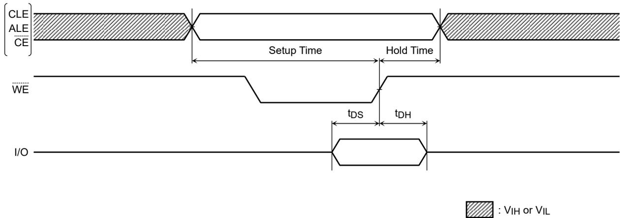
Command Input Cycle Timing Diagram
