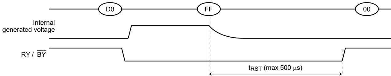
When a Reset (FFh) command is input during Read operation
