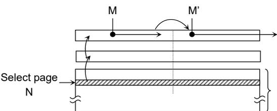
During the serial data output from the Data Cache, the column address can be changed by inputting a new column address using the 05h and E0h commands. The data is read out in serially starting at the new column address. Random Column Address Change operation can be done multiple times within the same page.
