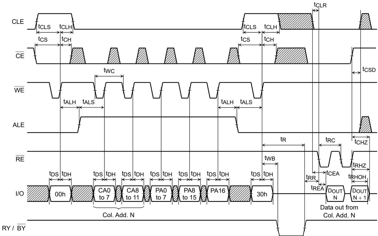
Read Cycle with Data Cache Timing Diagram (2/2)
