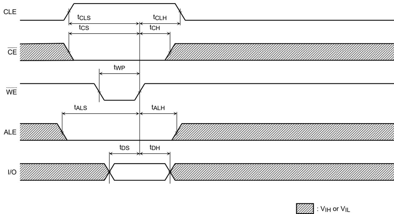
Address Input Cycle Timing Diagram
