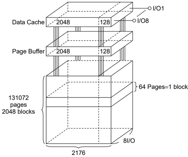
A page consists of 2176 bytes in which 2048 bytes are used for main memory storage and 128 bytes are for redundancy or for other uses.
