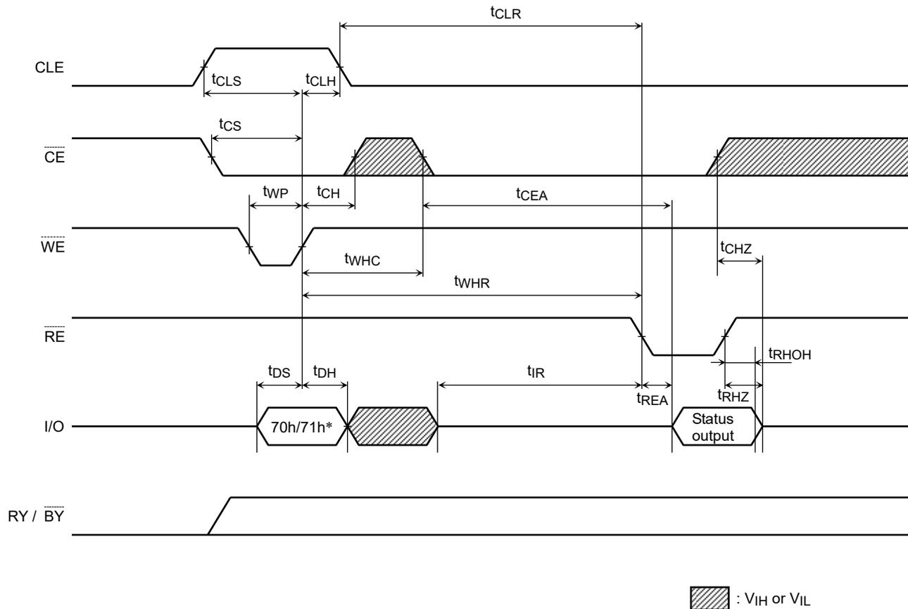
Read Cycle Timing Diagram
