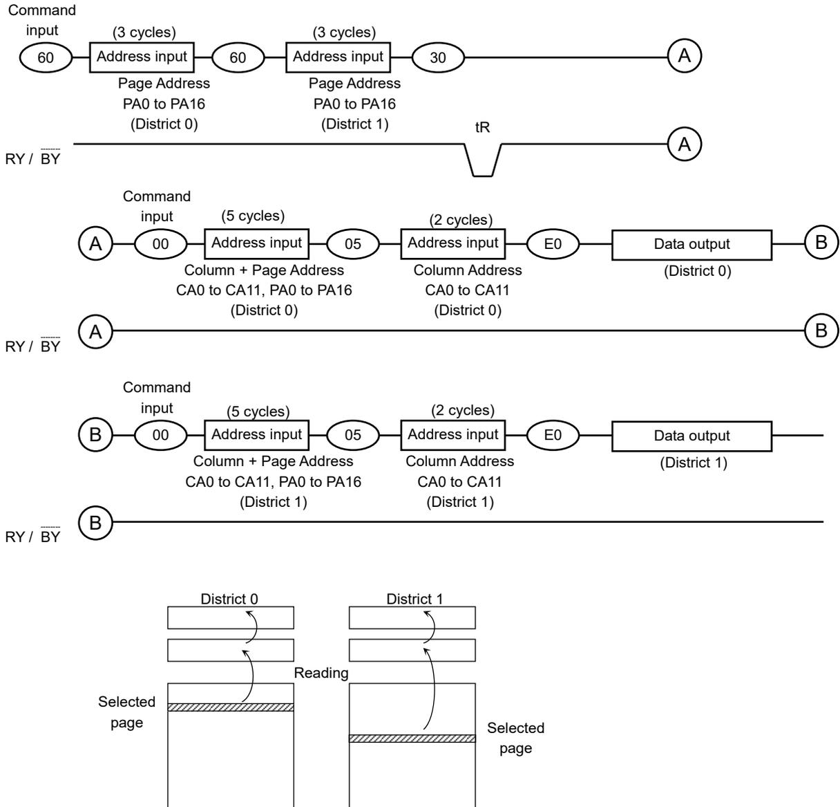
The data transfer operation from the cell array to the Data Cache via Page Buffer starts on the rising edge of  $\overline{WE}$  in the 30h command input cycle (after the 2 Districts' address information has been latched). The device will be in the Busy state during this transfer period.
