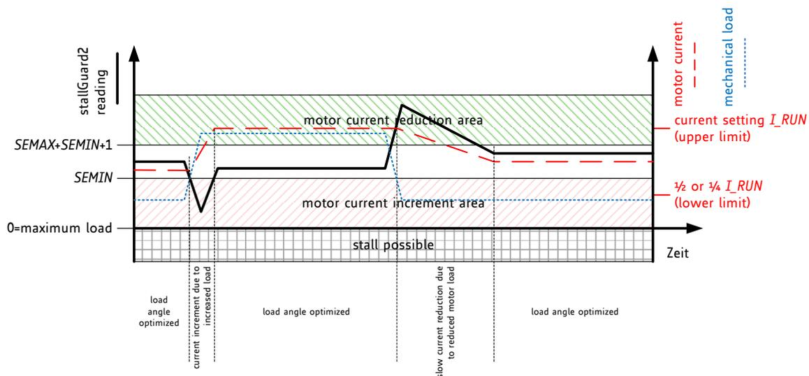
**Figure 12.1** CoolStep adapts motor current to the load
