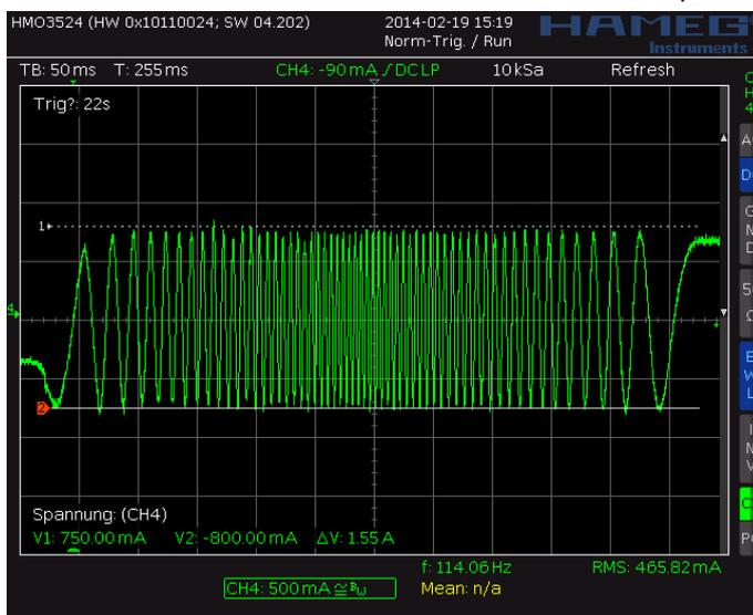
Figure 7.2 Scope shot: good setting for  $PWM\_GRAD$
