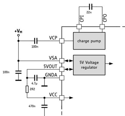
Figure 3.4 RC-Filter on VCC for reduced ripple
