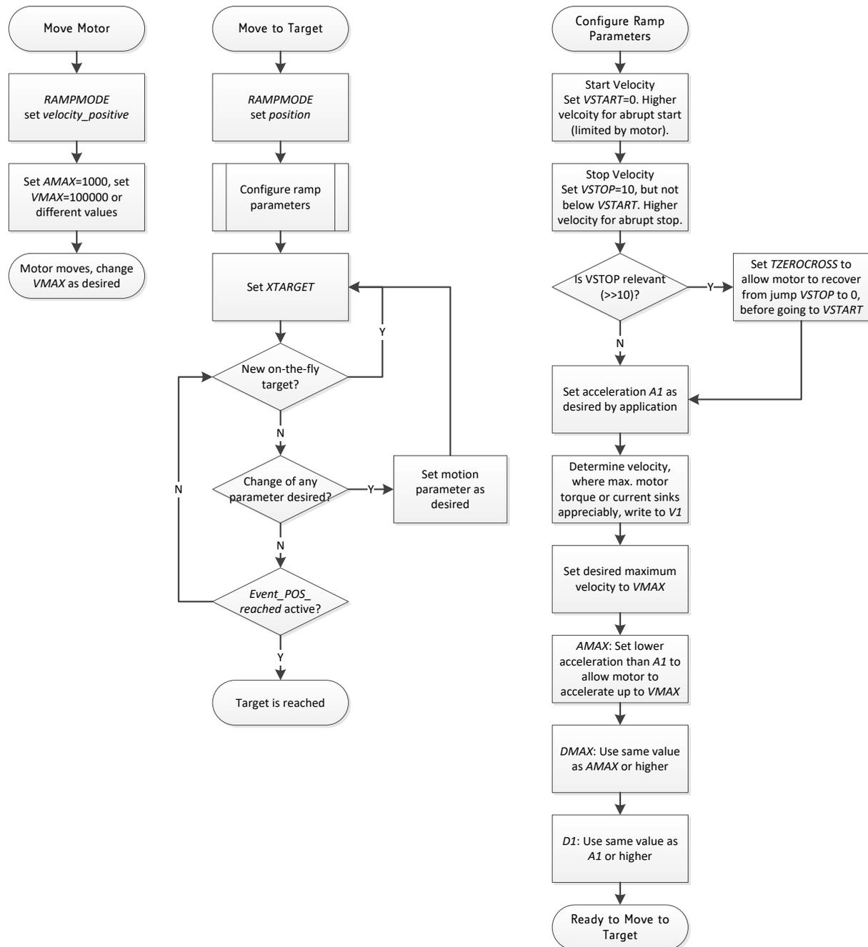
**Figure 14.3** Moving the motor using the motion controller
