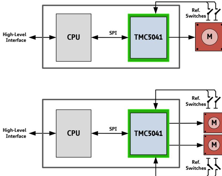
Two reference switch inputs can be used for each motor. A single CPU controls the whole system, which is highly economical and space saving, because the TMC5041 covers all functionality required to drive the motor.
