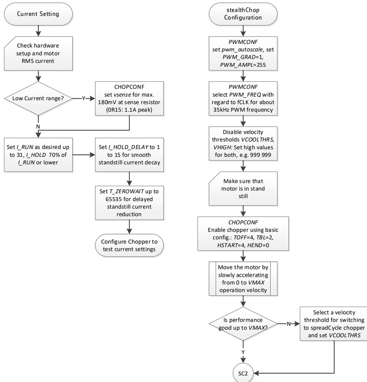
Figure 14.1 Current setting and first steps with StealthChop
