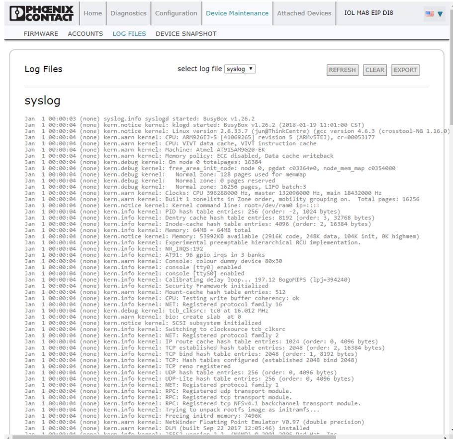
Figure 5-31 syslog file displayed on the “Log Files” page
