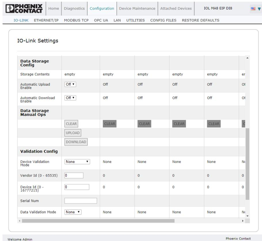
Figure 5-9 “Data Storage Config” options on “IO-Link Settings” page
