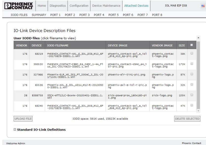
Figure 5-33 “IO-Link Device Description Files” page
