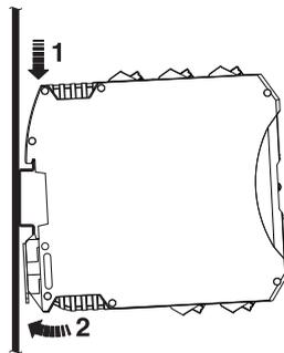
Figure 3-1 DIN rail mounting
