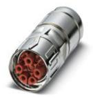
Cable connector, straight long, shielded: yes, SPEEDCON locking, M40, No. of pos.: 4+4+4+PE / 3+N+PE, type of contact: Socket, Crimp connection, cable diameter range: 9 mm ... 14 mm
