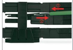
All distribution connector connections are locked and protected against accidental disconnection directly after mating. Locking of any connection is released using a screwdriver, even if all connections are used.
