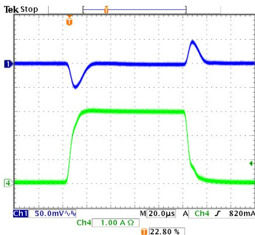
Load transient, 0 – 3A,  $V_{IN}/V_{OUT} = 5.5V/1.2V$
