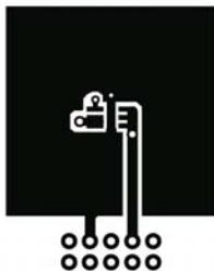
a)  $60^\circ\text{C/W}$  when mounted on a  $1\text{ in}^2$  pad of 2 oz copper
