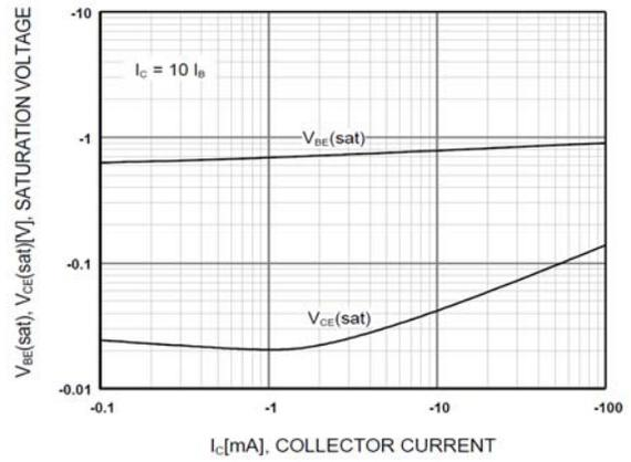
Figure 2. Base-Emitter Saturation Voltage Collector-Emitter Saturation Voltage
