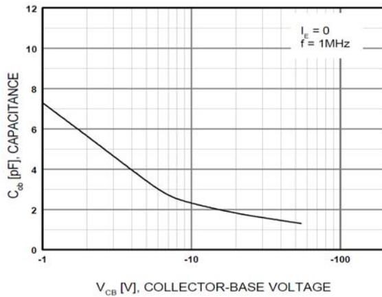
Figure 3. Output Capacitance
