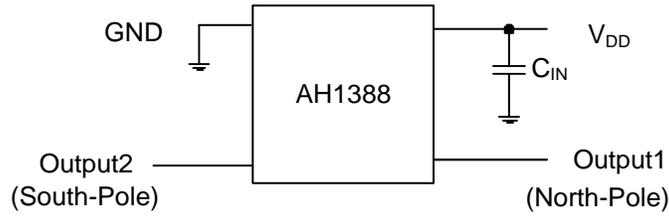
Note: 4.  $C_{IN}$  is for power stabilization and to strengthen the noise immunity, the recommended capacitance is 100nF typical and should be placed as close to the supply pin as possible.
