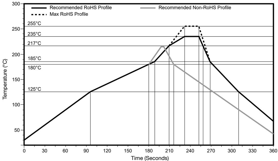
Figure 11. Solder Profile for the ANT-915-VHETH Antenna
