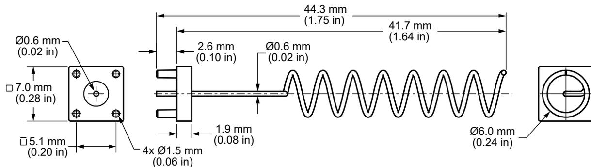
Figure 1. ANT-915-VHETH Antenna Dimensions
