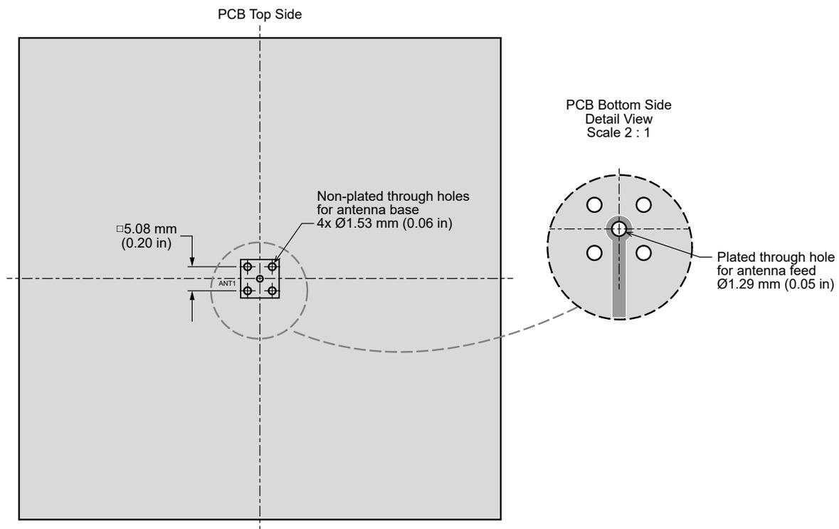
Figure 10. ANT-915-VHETH Antenna Placement on PCB
