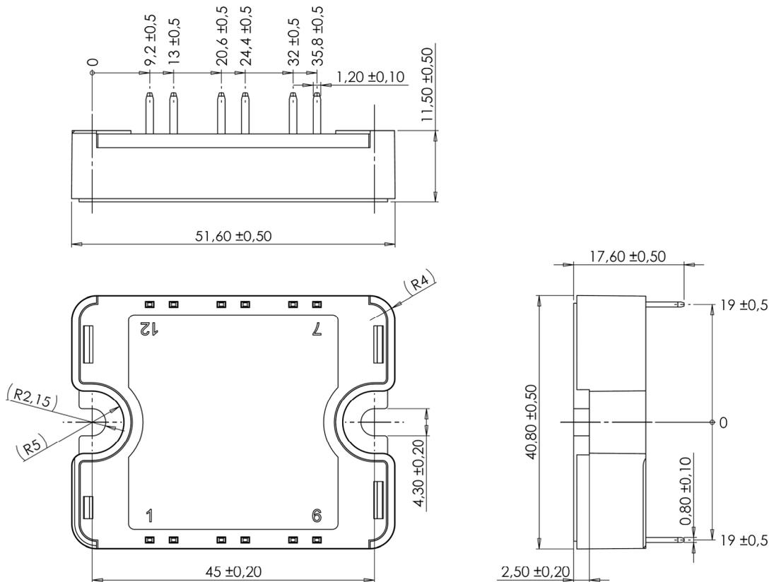
See application note 1904 - Mounting Instructions for SP1 Power Modules on [www.microsemi.com](http://www.microsemi.com)
