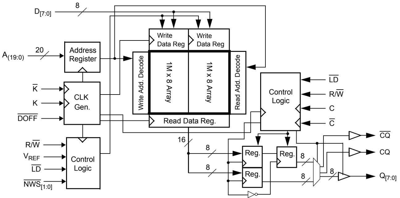
**Logic Block Diagram – CY7C1393KV18**
