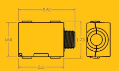
Use the ILLUMRA™ CUV Control Extender to wirelessly bridge control from one circuit to another. The Control Extender monitors any line voltage circuit and broadcasts the status to wirelessly control one or more circuits connected to compatible receivers.
