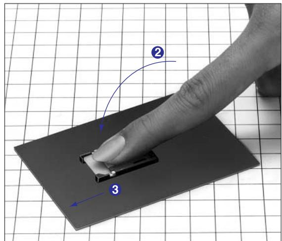
Close the card holder, press the slider, and at the same time move it in the direction marked "LOCK" on the card holder. A click sound will indicate that the lock has been engaged.
