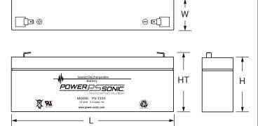
**L**: 7.00 (178) **W**: 1.37 (35) **H**: 2.36 (60) HT: 2.59 (66) Tolerances are +/- 0.04 in. (+/- 1mm) and +/- 0.08 in. (+/- 2mm) for height dimensions.
