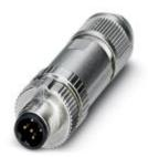
Bus system connector, INTERBUS (500 kbps), 5-position, shielded, Plug straight M12, B-coded, Push-in connection, knurl material: Zinc die-cast, nickel-plated, external cable diameter 4 mm ... 8 mm
