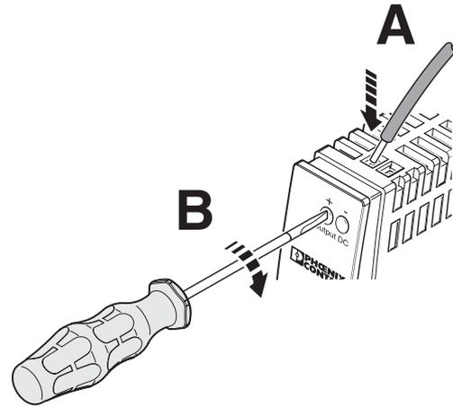
Figure 8 Connecting cables
