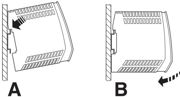
Figure 3 Mounting on a DIN rail
