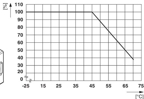
Rotated mounting position 180° X-axis
