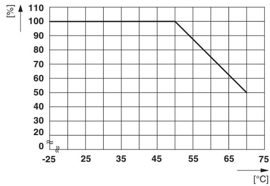
Rotated mounting position 270° Z-axis
