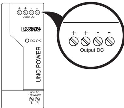
Figure 7 Screw connection for output DC +/-
