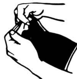
11. Snip off corner of "Unipak" container and pour Compound into Barrel (through opening for inline splice, through upper end for butt splice) until completely full.
