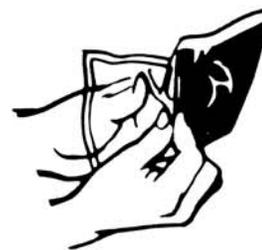
Thoroughly mix by squeezing Compound back and forth 30 to 40 times. Strip Compound from corners while mixing.
