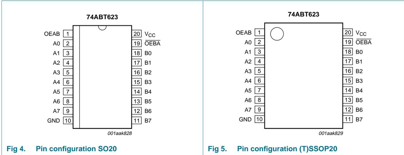
Fig 4. Pin configuration SO20
