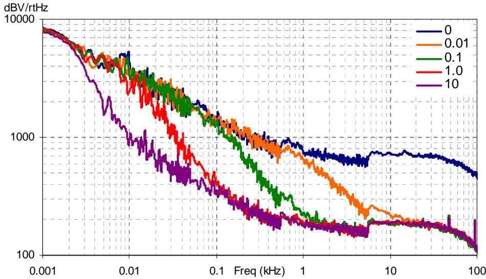
Figure 3-8. Typical AGND Noise with P2[4] Bypass
