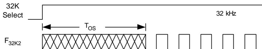
Figure 3-4. External Crystal Oscillator Startup Timing Diagram
