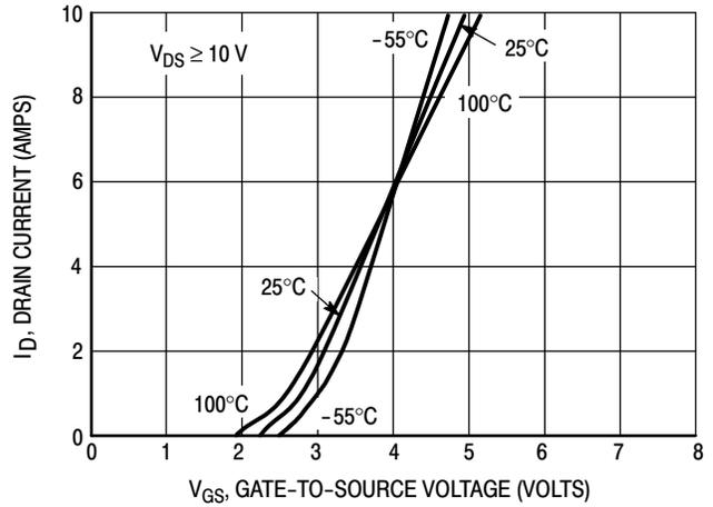
Figure 2. Transfer Characteristics
