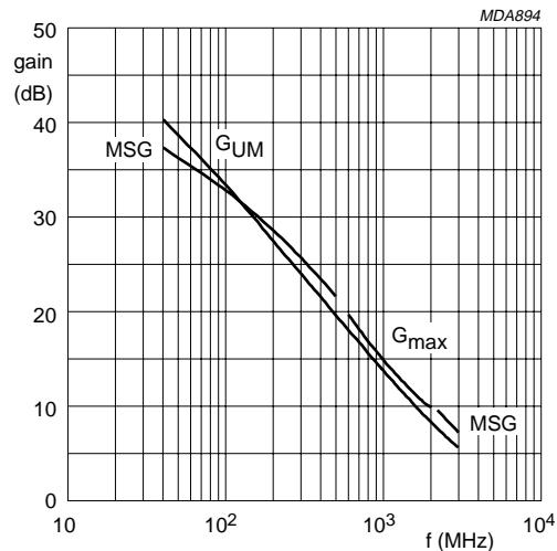
$I_C = 30 \text{ mA}; V_{CE} = 6 \text{ V.}$
