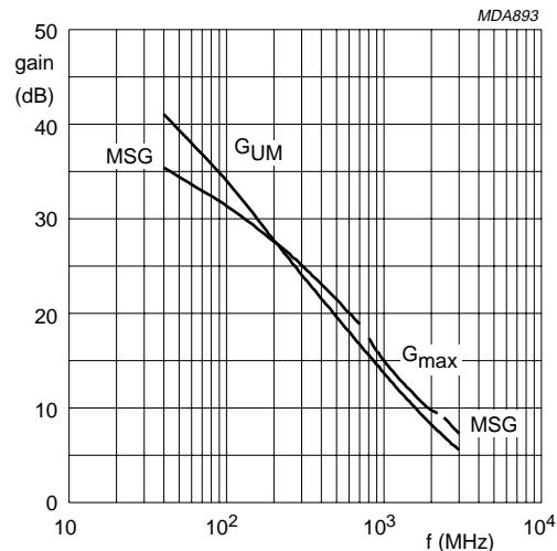
$I_C = 15 \text{ mA}; V_{CE} = 6 \text{ V.}$
