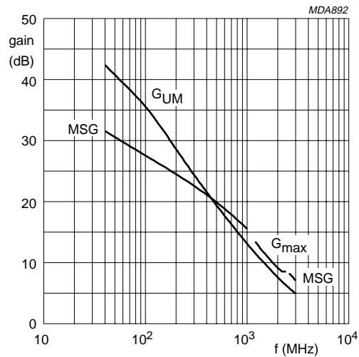
$I_C = 5 \text{ mA}; V_{CE} = 6 \text{ V.}$
