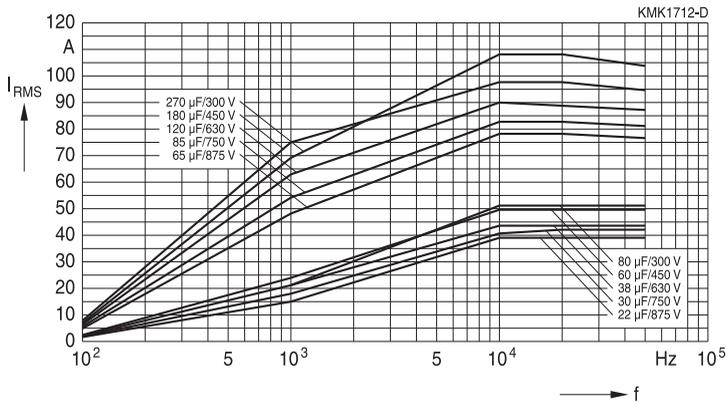
Curves characteristics ( $I_{RMS}$  derating versus temperature)
