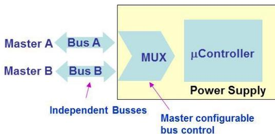
Diagram showing the dual I<sup>2</sup>C bus system.
