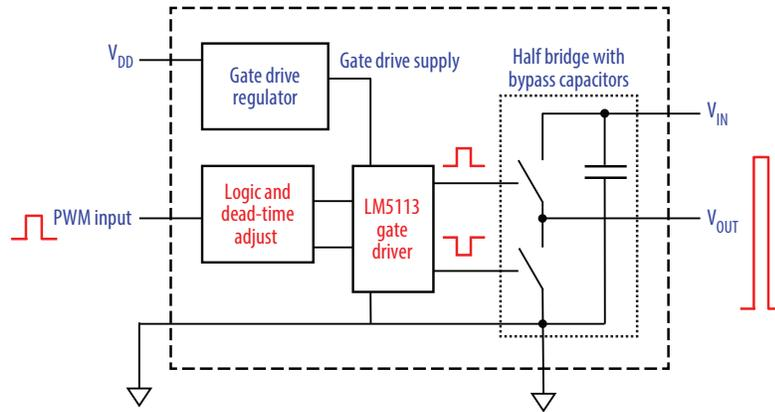
Figure 1: Block diagram of EPC9085 development board
