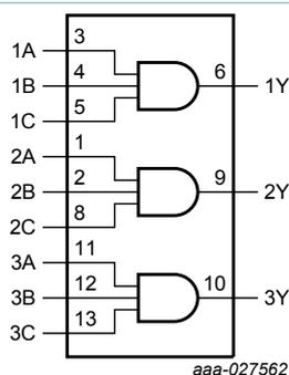
Figure 1. Functional diagram
