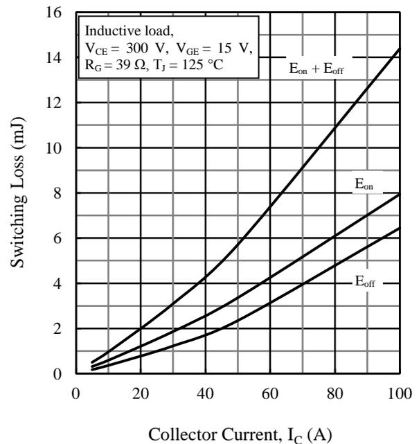
Figure 17. Switching Loss vs. Collector Current
