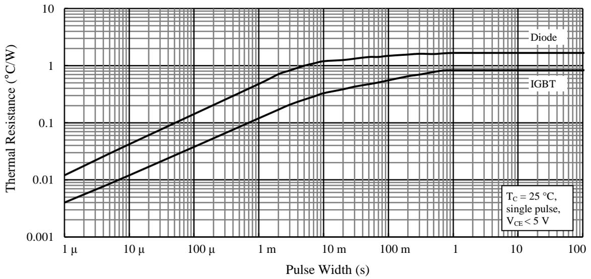
Figure 21. Transient Thermal Resistance
