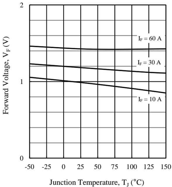
Figure 20. Diode Forward Voltage vs. Junction Temperature
