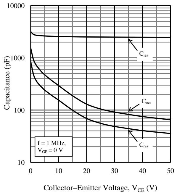
Figure 11. Capacitance Characteristics
