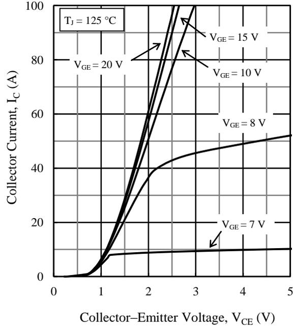
Figure 7. Output Characteristics ( $T_J = 125\text{ }^\circ\text{C}$ )
