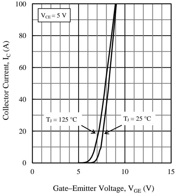
Figure 8. Transfer Characteristics
