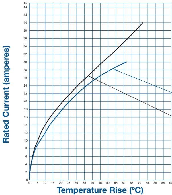
Temperature curve developed using **PCIC16W7M400A1** and **PCIC16W7F9300A1** connectors and 12 AWG wire. All size 16 contacts under load.
