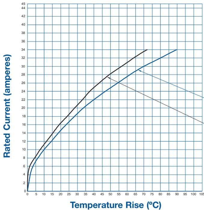
Temperature curve developed using **PCIB26W11M400A1** and **PCIB26W11F9300A1** connectors and 12 AWG wire. All size 16 contacts under load.
