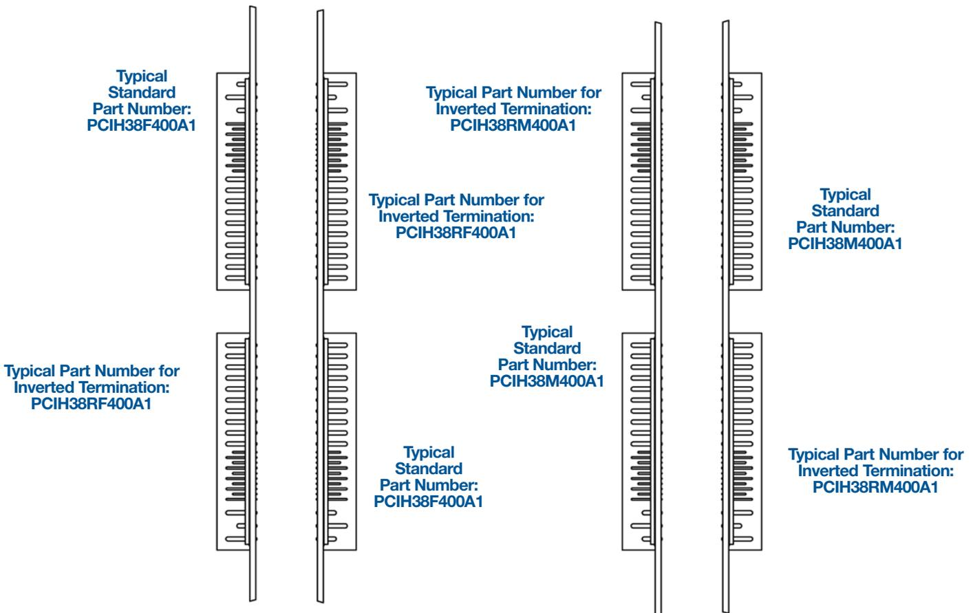
Inverted termination options allow flexibility in positioning the connector as best suited for specific applications.
