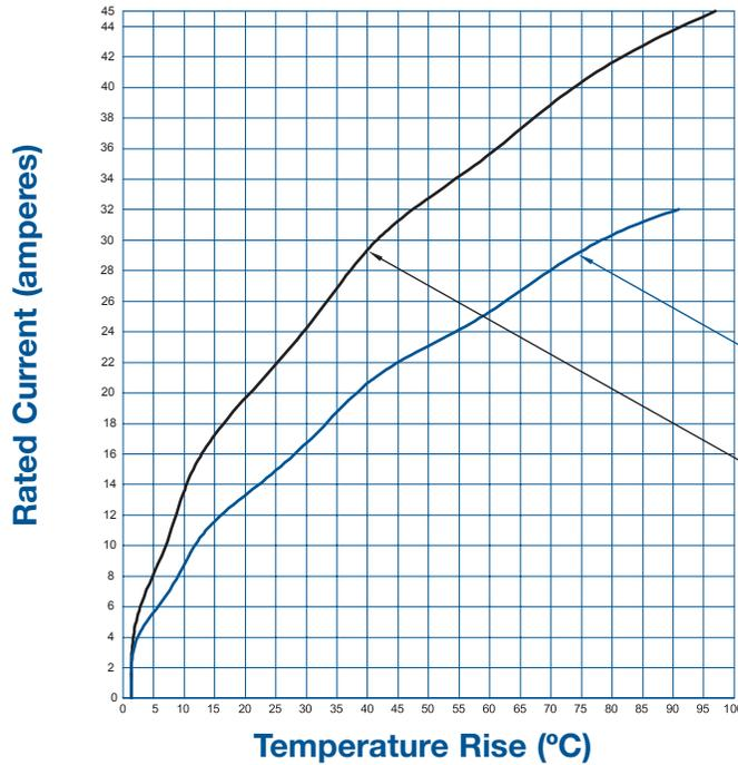
Temperature curve developed using **PCIM30W15M400A1** and **PCIM30W15F9300A1** connectors and 12 AWG wire. All size 16 contacts under load.
