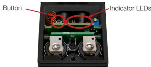
5. If the indicator LEDs do not automatically begin flashing, turn on the sensor by pressing and holding the button for five seconds until the LED to the right of the button flashes.
