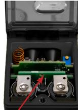
3. Insert the AA lithium batteries and verify the positive and negative terminals of each battery align to the positive and negative terminals. Caution: There is risk of damage if the batteries are installed incorrectly.
