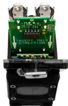
4. Slide the battery board back into the housing.
