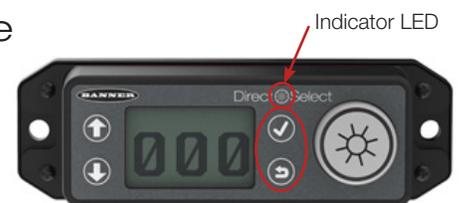
3. If the indicator LED does not automatically begin flashing, turn on the Operator Interface by pressing and holding the up and down arrow buttons together for five seconds or until the small light starts flashing red.
