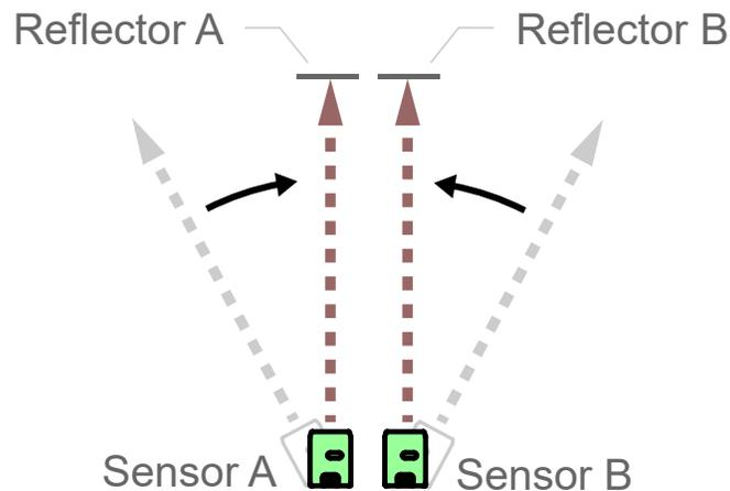
Note: From behind the Sensor Pair, Sensor A may be either to the left or to the right of Sensor B. This will depend on whether the Sensor Pair is mounted on the left or the right of a door. The alignment process will be the same for either position.
