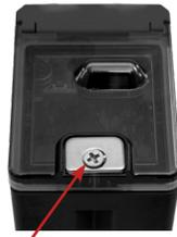
2. Using a small Phillips screwdriver, insert the tip into the small hole in the battery holder and pry up the battery holder. Slide the battery board up and out of the housing.
