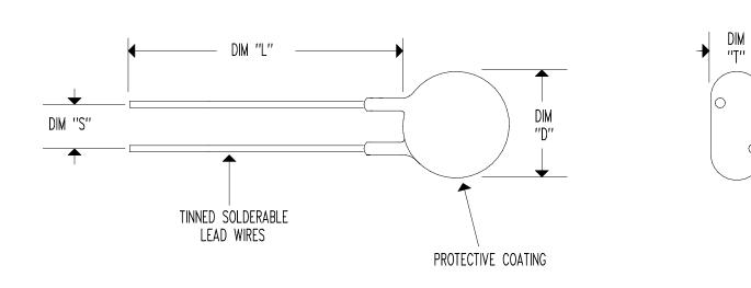
RESISTANCE @  $\pm 25$ 'C = 5  $\Omega$   $\pm$  20% MAXIMUM STEADY STATE CURRENT = 14 AMPS RESISTANCE @ MAXIMUM CURRENT = 0.060  $\Omega$  NOMINAL
