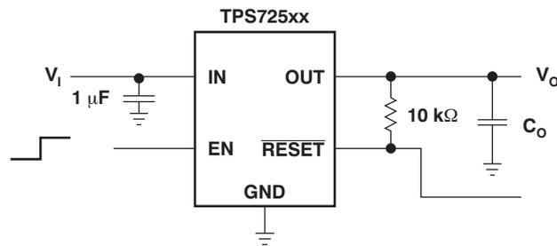
Figure 19. TPS72501 Fixed Output Typical Application Diagram
