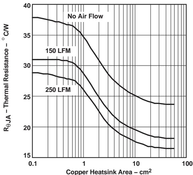
Figure 21. DPAK Thermal Resistance vs Copper Heatsink Area
