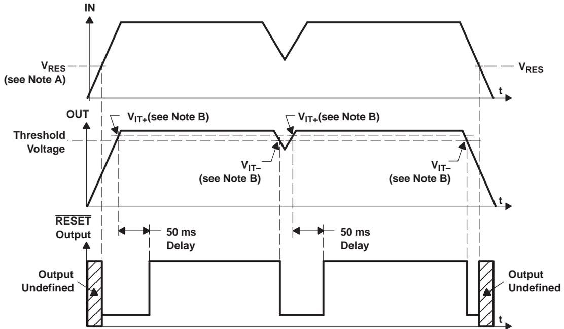
NOTES: A.  $V_{RES}$  is the minimum input voltage for a valid RESET. The symbol  $V_{RES}$  is not currently listed within EIA or JEDEC standards for semiconductor symbology.
