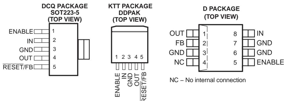
NOTE: TPS72501 replaces RESET with FB. Tab is GND for the DCK and KTT packages.
