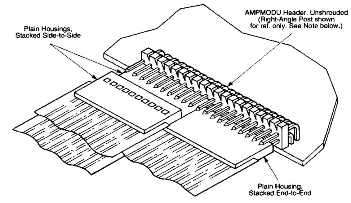
Note: Plain housings are side-to-side and end-to-end stackable on either straight or right-angle posted, unshrouded AMPMODU headers. Latch and detent styles are end-to-end stackable only.
