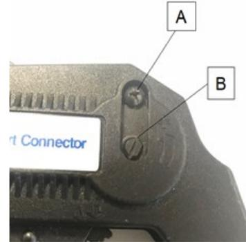
This Tool incorporates an eccentric axle and an adjustable wheel to adjust and recalibrate to ensure correct crimp performance. Should adjustment be necessary, the following procedure should be followed:
