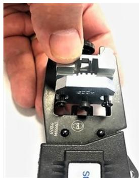
To remove the die set from the hand tool frame loosen thumb Screw (C) completely. Close Ratcheted tool handle one click to reveal the Cap head screw (D). With the opening (E) (approximately .28"), push the die set out from the opposite side.
