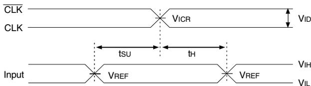
**Voltage Waveforms - Setup and Hold Times**
