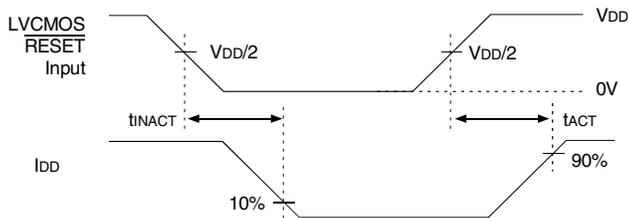
**Voltage and Current Waveforms
