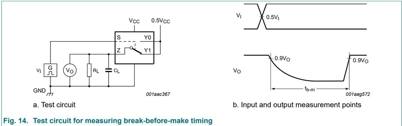
Fig. 14. Test circuit for measuring break-before-make timing
