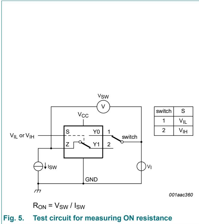
Fig. 5. Test circuit for measuring ON resistance
