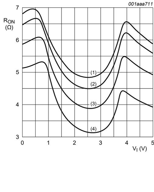
Fig. 11. ON resistance as a function of input voltage;  $V_{CC} = 5.0\text{ V}$
