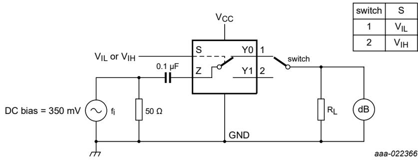
Adjust  $f_i$  voltage to obtain 0 dBm level at output. Increase  $f_i$  frequency until dB meter reads -3 dB.
