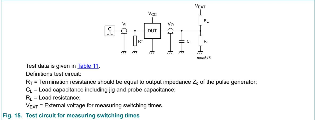
Fig. 15. Test circuit for measuring switching times
