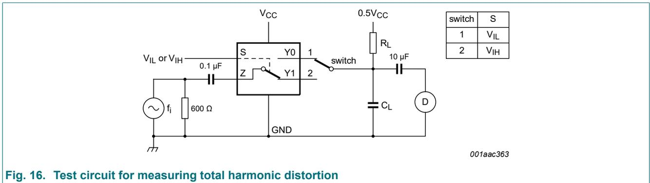
**Fig. 16. Test circuit for measuring total harmonic distortion**
