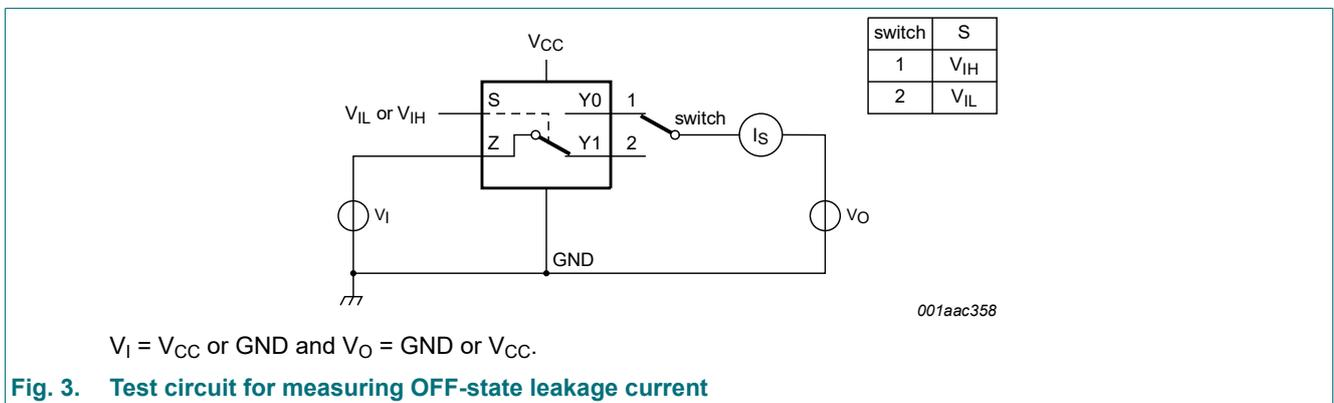
**Fig. 3. Test circuit for measuring OFF-state leakage current**
