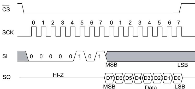
Figure 8. Write Status Register (WRSR) Instruction Timing
