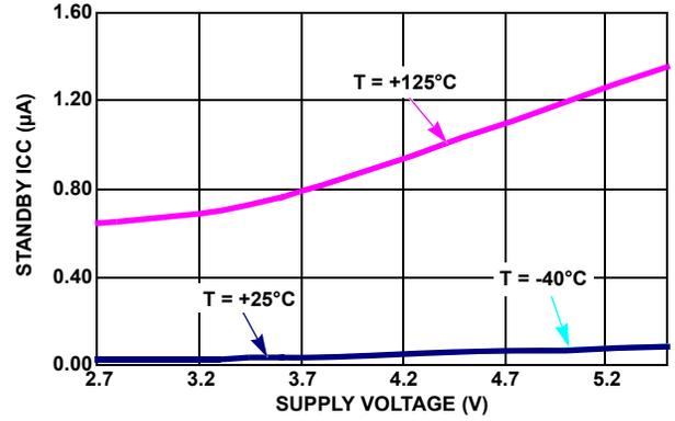
FIGURE 2. STANDBY I<sub>CC</sub> vs V<sub>CC</sub>
