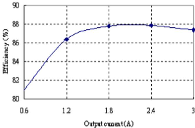
**Figure 3:** Converter efficiency vs. output current
