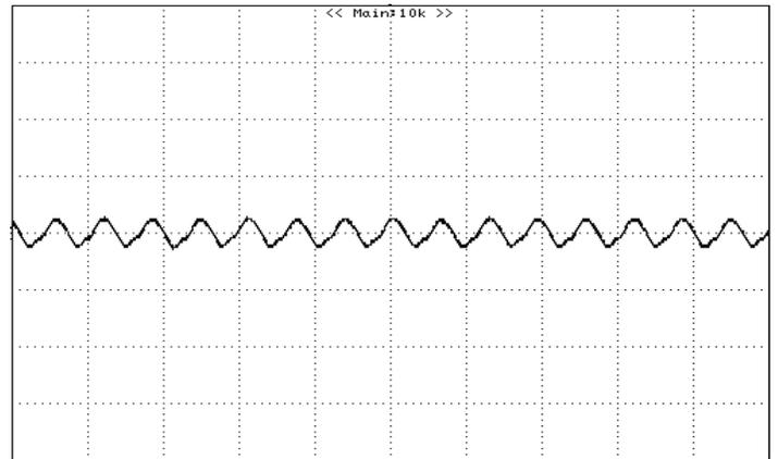
**Figure 8:** Output ripple & noise at 12Vin, 2.5V/3A out
