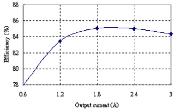
**Figure 4:** Converter efficiency vs. output current
