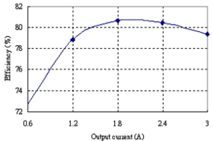
**Figure 6:** Converter efficiency vs. output current
