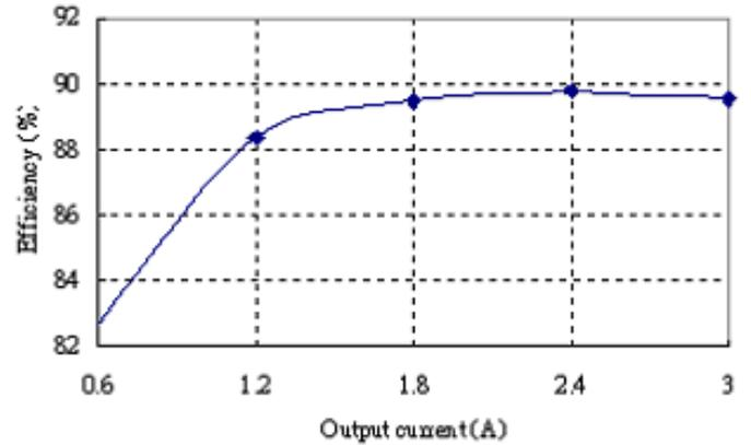
**Figure 2:** Converter efficiency vs. output current
