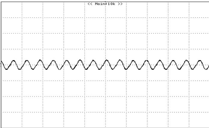
**Figure 9:** Output ripple & noise at 12Vin, 3.3V/3A out
