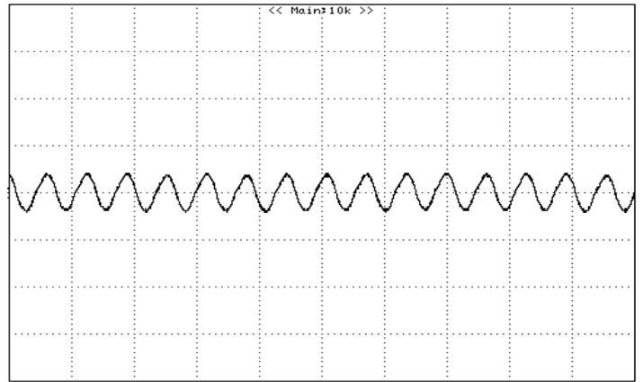
**Figure 10:** Output ripple & noise at 12Vin, 5.0V/3A out
