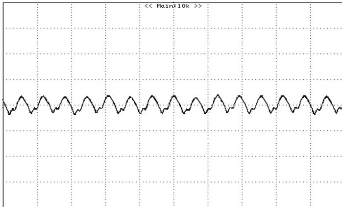
**Figure 7:** Output ripple & noise at 12Vin, 1.2V/3A out
