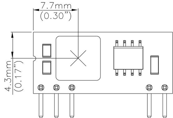
Figure 28: Temperature measurement location
