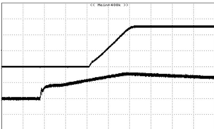
**Figure 11:** Turn on delay time at 12vin, 5.0V/3A out (2mS/div)
