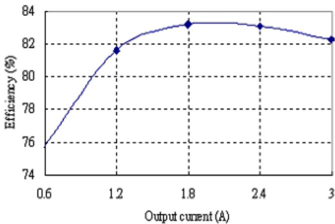
**Figure 5:** Converter efficiency vs. output current
