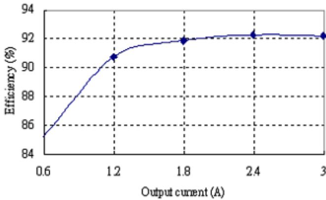
**Figure 1:** Converter efficiency vs. output current
